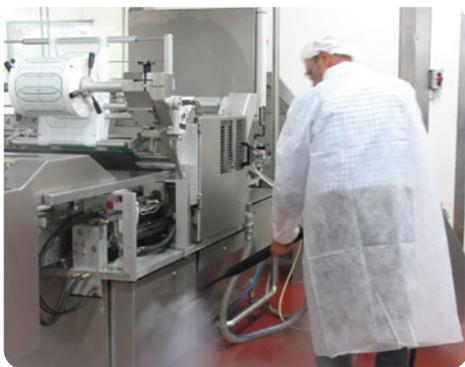
Blast food residues off processing equipment and preparation areas with 150 bar high pressure water and then thermally sanitise using +180°C super heated 94% dry system.
