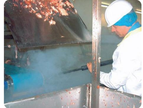
The STEAM PRESSURE is ideal for use in environments like abattoirs where the high pressure water rids surfaces of meat/bone residue in seconds and the +180°C melts fats and sanitises.
