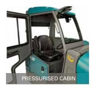
Operate safely and comfortably in the most severe environments with an optional FOPS Certified (ISO 3449) pressurised cabin, available with air conditioning.
