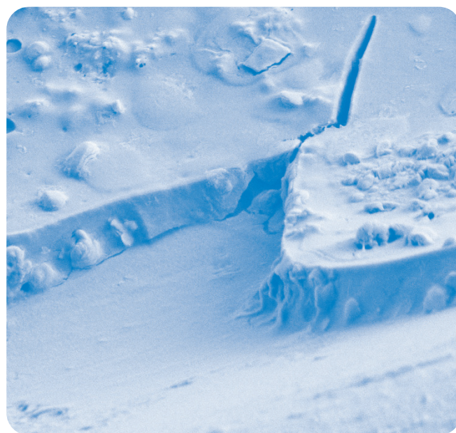
Encapsul8 polymer residue fracturing from carpet fibre surface.
