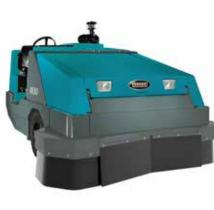
The 800 is the largest and most powerful machine in its class – designed to sweep heavy concentrations of industrial debris, pellets, rocks and glass found in the harshest industrial and manufacturing environments, both indoors and out.
