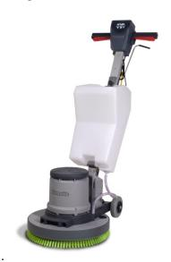
These machines are traditionally a basic corded machine, with a high torque motor producing a low-speed scrub head, which can either hold a brush or cleaning pad. These machines can come with or without a clean water tank, but do not usually come with a suction system or recovery tank to pick up the slurry. A wet vacuum or other method is often needed to complete the cleaning process.
