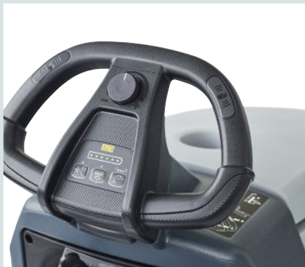
Ergonomic handle with touchpoints, One-Touch™ button and instruction stickers makes the machine simple for the operator to get started
